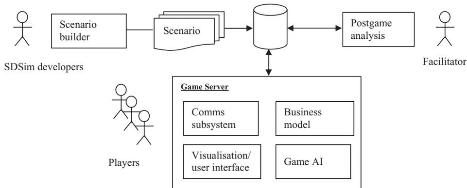
Figure 1: Internal subsystems of the SDSim game
